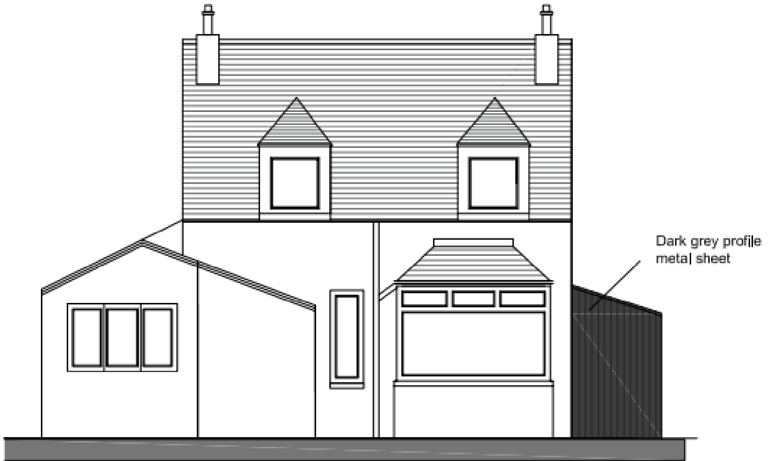
PROPOSED NORTH ELEVATION 1:100 - Unaltered
