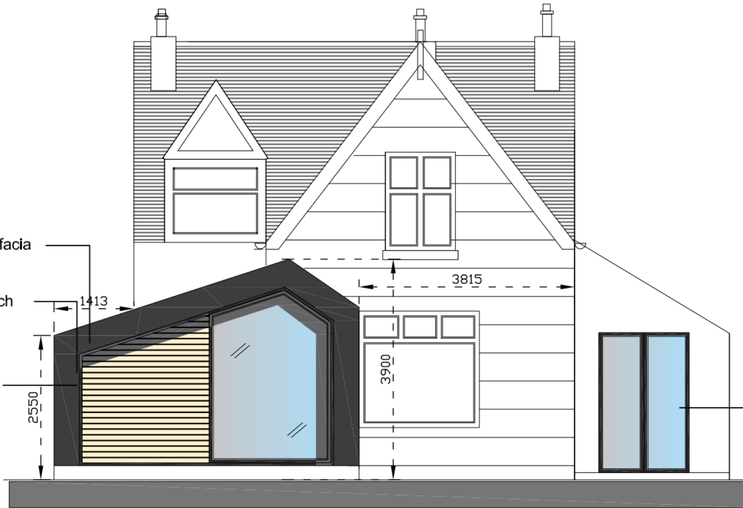
PROPOSED SOUTH ELEVATION 1:100
